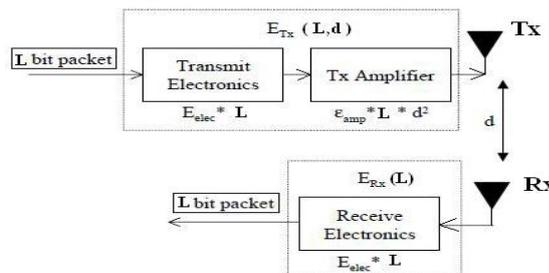
**Fig. 1.3** Radio Energy dissipation Model
